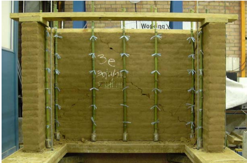
Figure 15a. Specimen 3E after simulation S8
