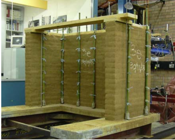
Figure 5a. Specimen 3E ready for testing. Note external vertical bamboo (inside and outside).
