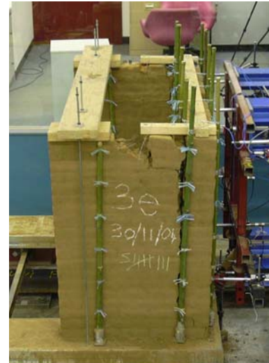
Figure 15b. Specimen 3E after simulation S8
