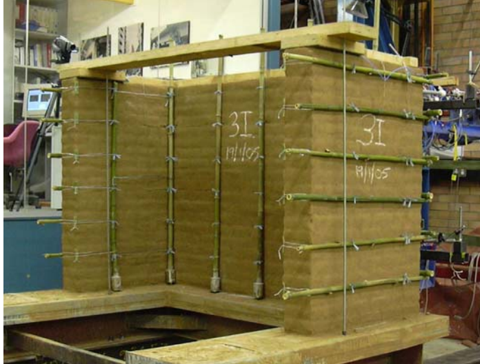
Figure 7a. Specimen 3I ready for testing. Note external horizontal bamboo (outside) and external vertical bamboo (inside).
