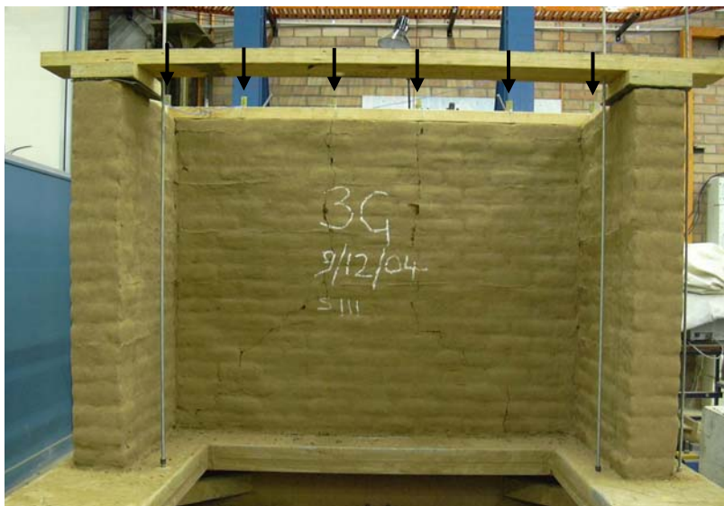
Figure 17a. Specimen 3G after simulation S3 (Arrows indicate the location of internal vertical bamboo)
