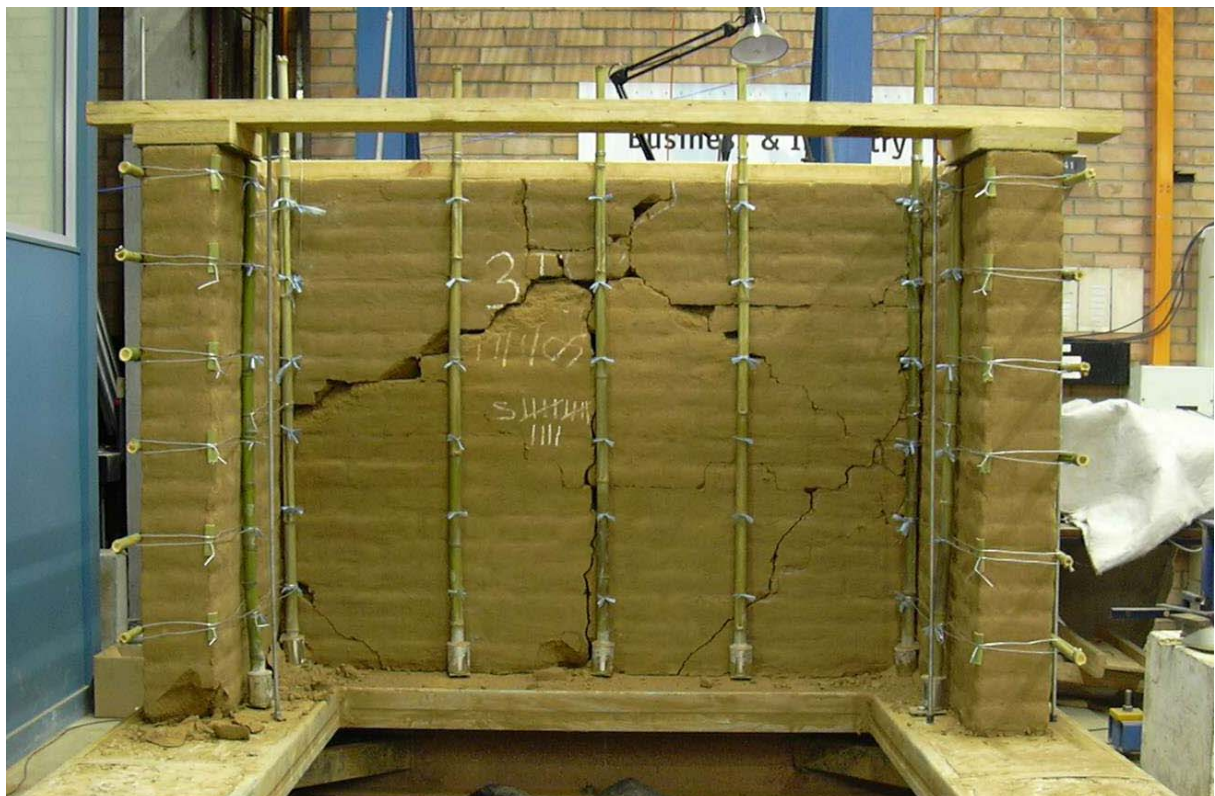
Figure 20. Specimen 3I after simulation S14
