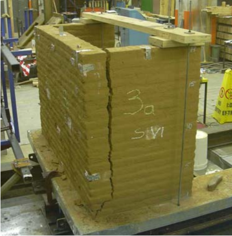
Figure 8. Large vertical crack in NW corner.
